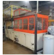
Nissei Model PF6-2B PET Stretch Blow Molding Machine
