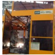
Nissei Model PF3-1BLL PET One Step Stretch Blow Molding Machine
