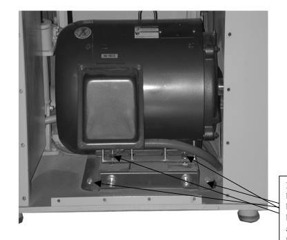
Loosen these 4 nuts on the bolts holding the unit on the base. Slide the motor either backwards or forwards to achieve the proper belt tension and retighten the nuts.
