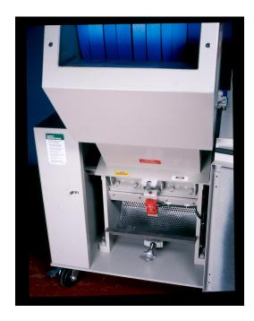
Opening the front latch allows access into chamber area. The pivoting door is allowed to swing open giving fast, and easy access to the major components.
