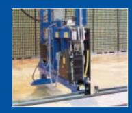
**KSR-2 Strapping Head.** Extremely reliable strapping head saddled in a carriage device, employs a double-tensioning feature to apply evenly distributed force around the entire load. The high-speed, all-electric, KSR-2 friction-seal strapping head has been proven in hundreds of industrial installations and produces a highly efficient seal joint.
